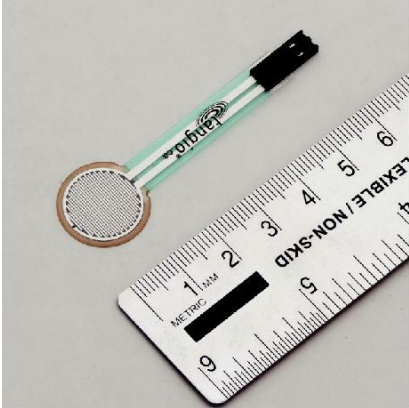
Figure 5. Example of a single-point sensor (WPE-503)
