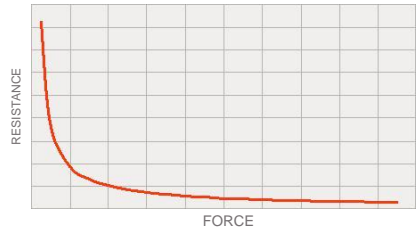
Figure 1. Typical FSR Force vs Resistance
