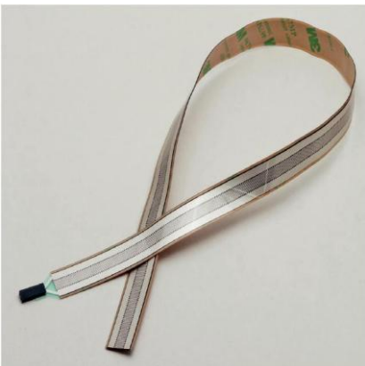
Figure 7. Example of a single-point sensor (WPE-508)
